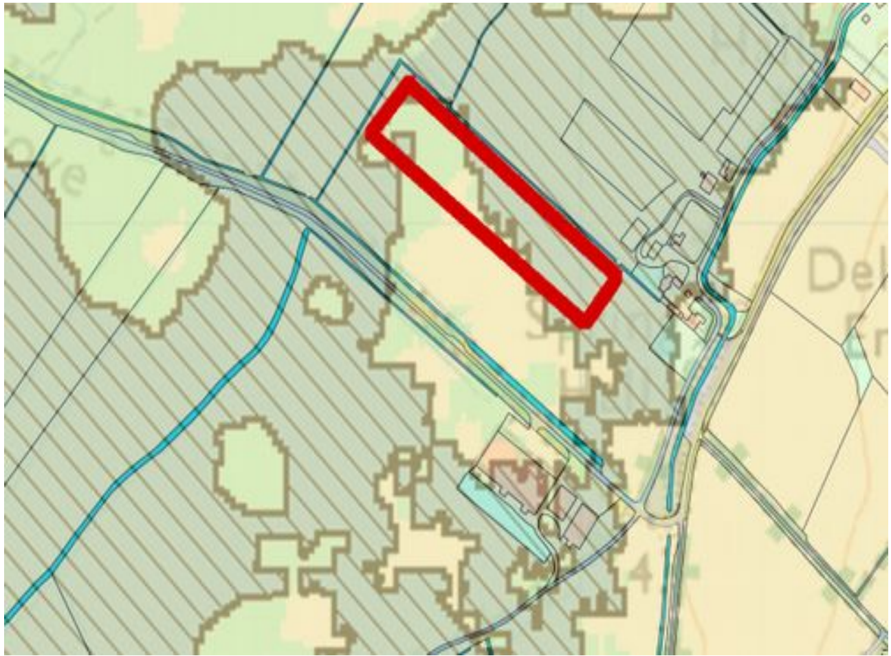
Figure 3: Site plan with flood map overlay. The boundary of the region covered by solar panels is shown in red. Light blue is flood zone two, dark blue is flood zone three. The hatching indicates that the area is protected by flood defences.
