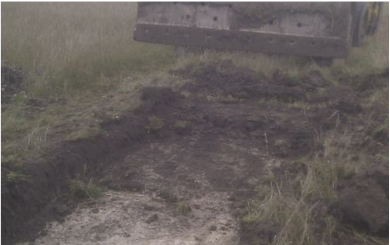
Figure 6: Soil characteristics. The clay subsoil is covered with well-drained topsoil throughout the site.
